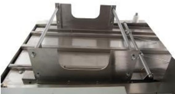
Thanks to Automatic Tray Feeding System that allows to run the machine with the single person. Just fill the storage with the trays than wait for the filled trays. Fully automated tray loading system for entrance or tray loading system onto trolley can be adapted to the machine on request. By the way system automatically fill trays, position the trays on trolleys.
