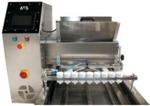
LCD touchscreen panel allows to user to control all the parameters of the machine such as length, height of the product, capacity, color ratio, speed etc. English and Russian language is available for control panel.
